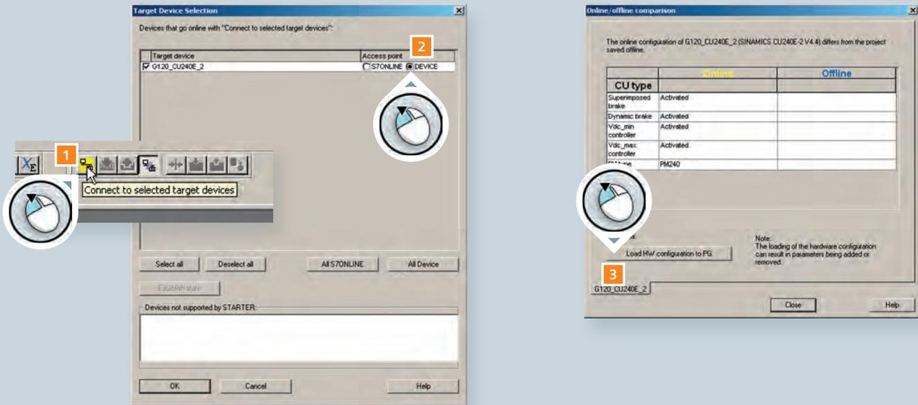
Now the converter data is loaded into the project and an online connection between PC and converter is established.
